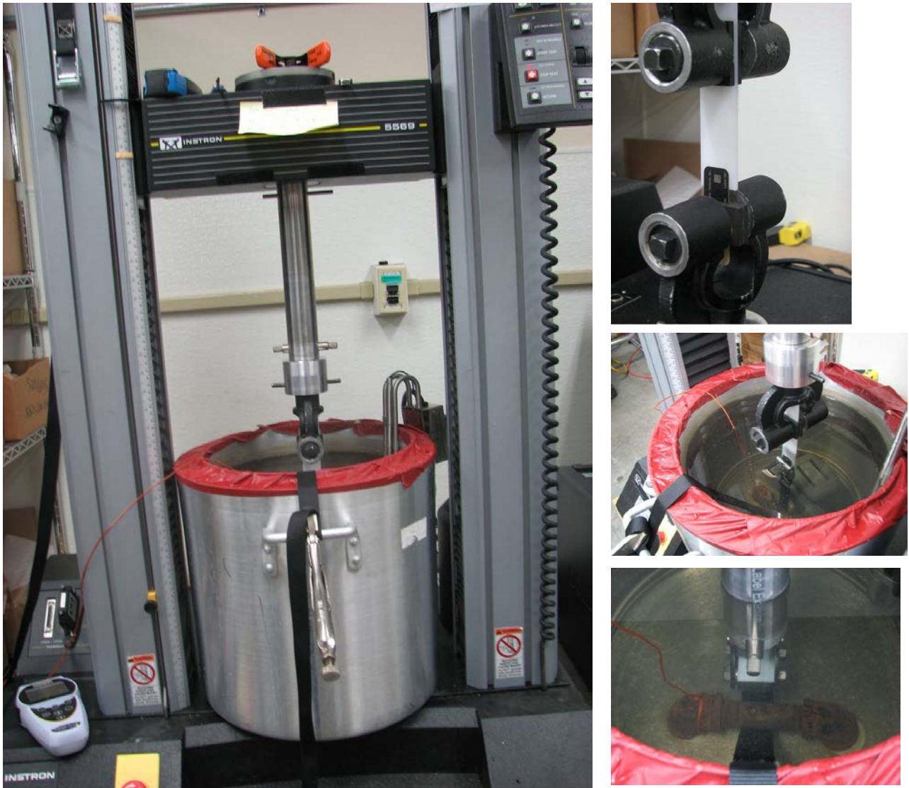
Figure 8. Left - Instron with heated water bath and clamped nylon strap. Right top - Air shear test. Right middle - Heated shear with added weights immersed in water to accommodate higher shear forces and unattached part of label bent to accommodate clamp. Right bottom - Heated peel test with visible orange thermocouple to monitor water temperature, floating roller peel fixture with white polypropylene test plate, and bottom fixed fixture epoxied to aluminum pot containing heated water.
