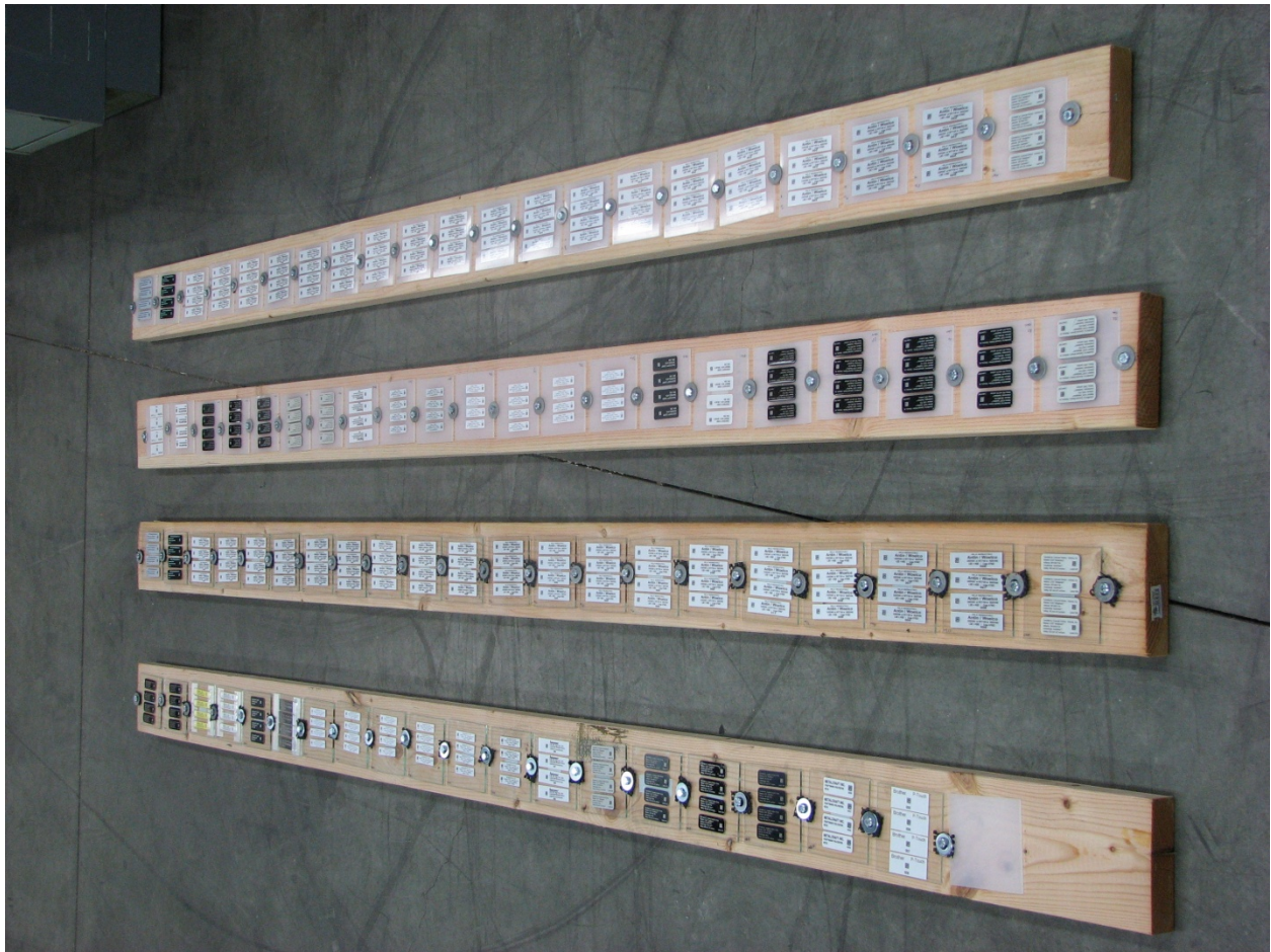
Figure 14. Labels attached to plates mounted on test boards for solar exposure testing
